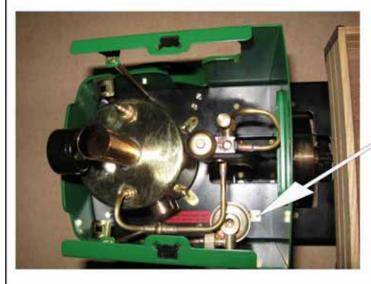
REMOVE FRONT ENGINE MOUNT SCREW AND FIT TANK IN POSITION SHOWN
