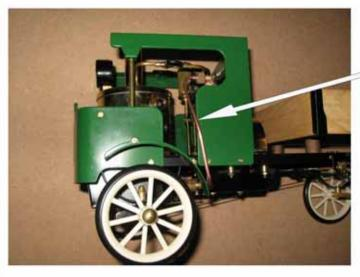
ASSEMBLE PIPE TO BURNER AS SHOWN BELOW, FIT BURNER INTO SLIDE IN BOILER FIRE BOX, CONNECT PIPE TO GAS TANK
