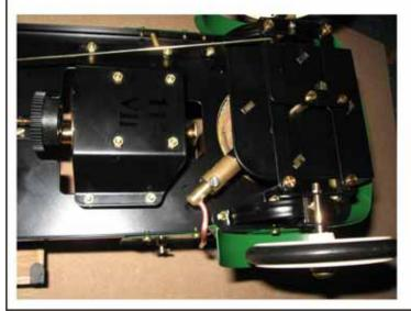
ENSURE BURNER IS CENTRAL UNDER BOILER, SOME ADJUSTMENT OF PIPE BENDS MAY BE NECESSARY,
