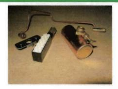
REMOVE RIGHT HAND SCREW, FIT BURNER INTO PLATE BUT DON'T TIGHTEN IN PLACE, SLIDE GAP IN PLATE INTO FIREBOX BULKHEAD
