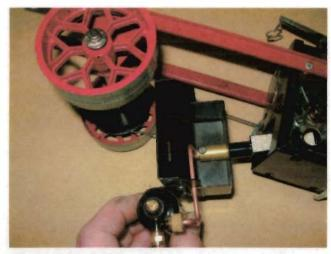
TURN THE UNIT THROUGH 90 deg. TO FIT INTO THE FIREBOX, AS SHOWN
