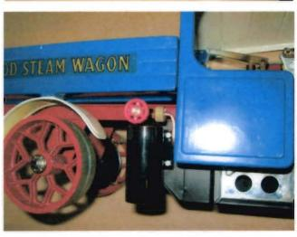
CHECK TANK VALVE IS TURNED OFF AND CONNECTION IS TIGHT, FILL TANK WITH GAS (BUTANE OR 70/30 BUTANE PROPANE MIX)
