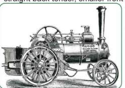
This sort of engine would be in general agricultural use, particularly working threshing machines and other equipment with a belt drive off the flywheel. There was a choice of power, this being the 7 nominal horse power version built in 1893.
