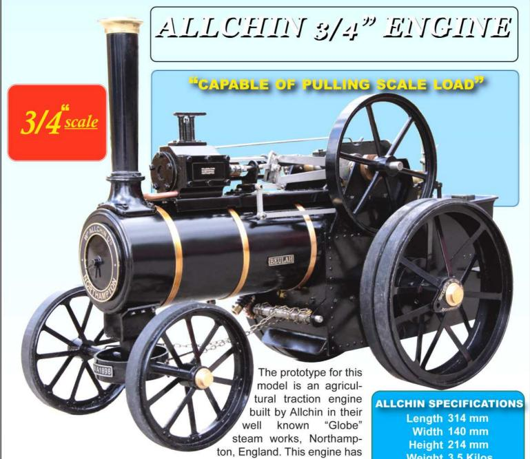
typical Victorian characteristics of the period, with a short smokebox, straight back tender, smaller front wheels and "dumpy" looking boiler.
